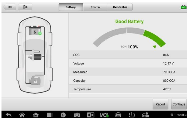
Figure 9-7 Battery Test Result Screen
