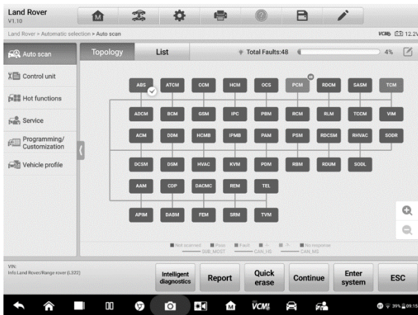
Figure 5-6 Sample Fault Scan on Topology Screen
