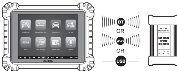
Figure 5-4 Tablet Connecting to the VCI
