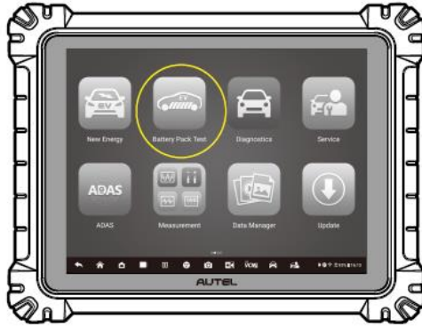
Figure 5-5 Tap Battery Pack Test
