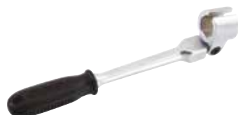
#818002 Oxygen sensor wrench - 6-pt wrench 22mm with flexible head - For easy mounting and removing of stuck oxygen sensors
